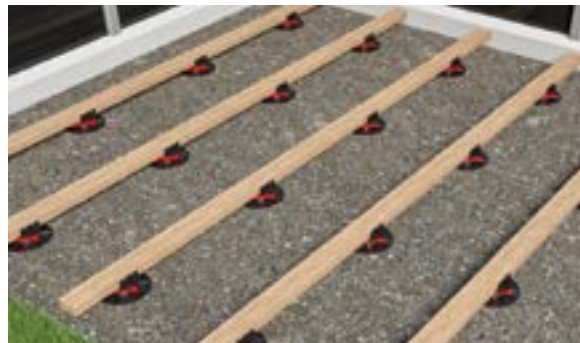
Place the pedestals on the ground, spacing them from 50 to 70 cm maximum
