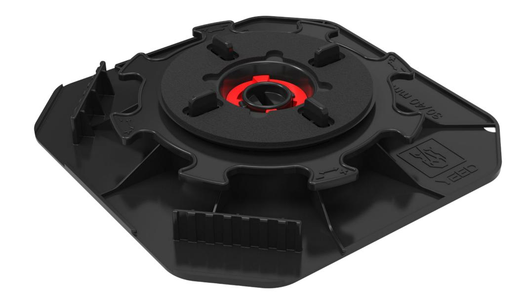
Discover the most efficient solution for any slab terrace installation. The UNIKA pedestal is height-adjustable from 30 to 40 mm. It can be raised to a height of up to 1 meter using the extension accessory. The height can be easily adjusted to the nearest millimeter using the adjustment ring: from the top by using the YEED Tightening key, or manually from the side.
