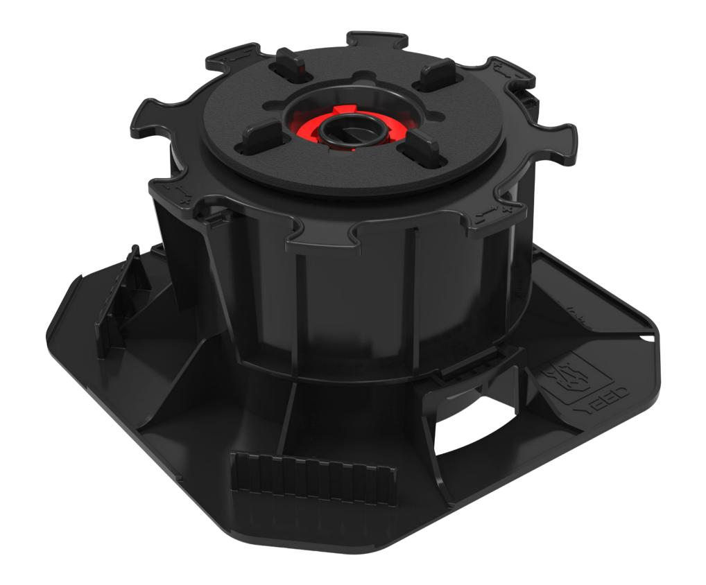
Discover the most efficient solution for any slab terrace installation. The UNIKA pedestal is height-adjustable from 40 to 60 mm. It can be raised to a height of up to 1 meter using the extension accessory. The height can be easily adjusted to the nearest millimeter using the adjustment ring: from the top by using the YEED Tightening key, or manually from the side.
